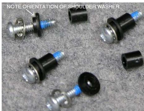
Note that the narrow side of the plastic shoulder washer goes toward the lock washer/screw head side
