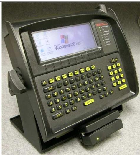
◀ LPA772 is a bracket for attaching a barcode or mag-stripe slot reader directly to the housing of the LANpoint 7 Data Collection Terminal. The slot reader is shown at the bottom of the terminal here, but it may be mounted at the top if desired.
