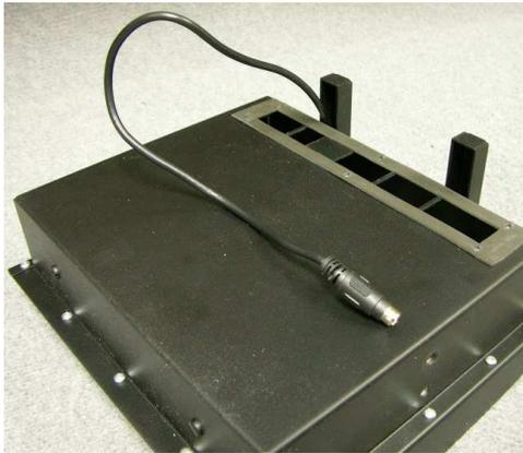
◀ Step 5: Position the bracket and loosely start the two black screws. Make sure the cable is routed through the slot reader bracket channel as shown and is not pinched
