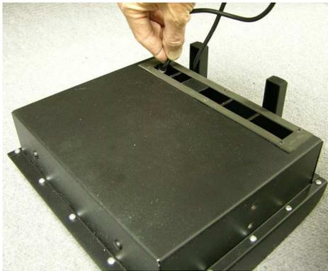
◀ Step 7: Align and insert the PS/2 slot reader plug into the right-hand side PS/2 connector that is labeled 'KEYBOARD'. Cable clearance is minimal but adequate.
