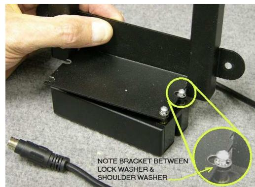
Note that the slot reader bracket separates the metal lock washer from the black nylon shoulder washer; be sure to orient the slot reader so that the read head (slim part of the body) is oriented properly (up or down) in relation to the badges to be read. In the example shown, the read head is pointing down because the badges to be used have the barcode printed on the face/front side of the card.
