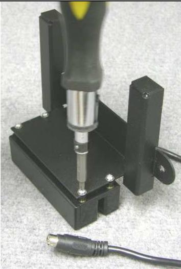
◀ Step 3: Install the remaining 2 screw sets and tighten them; the narrow shoulder of the black nylon shoulder washer will fit the width of the mounting slots in the bracket.
